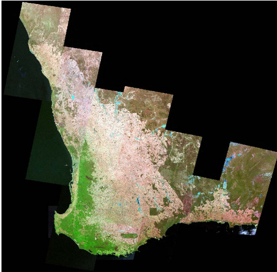
Figure 1: 2003 Landsat TM mosaic of the Western Australian agricultural area (bands 5,4,3 in RGB). The area shown is approximately 1000 km by 950 km.
