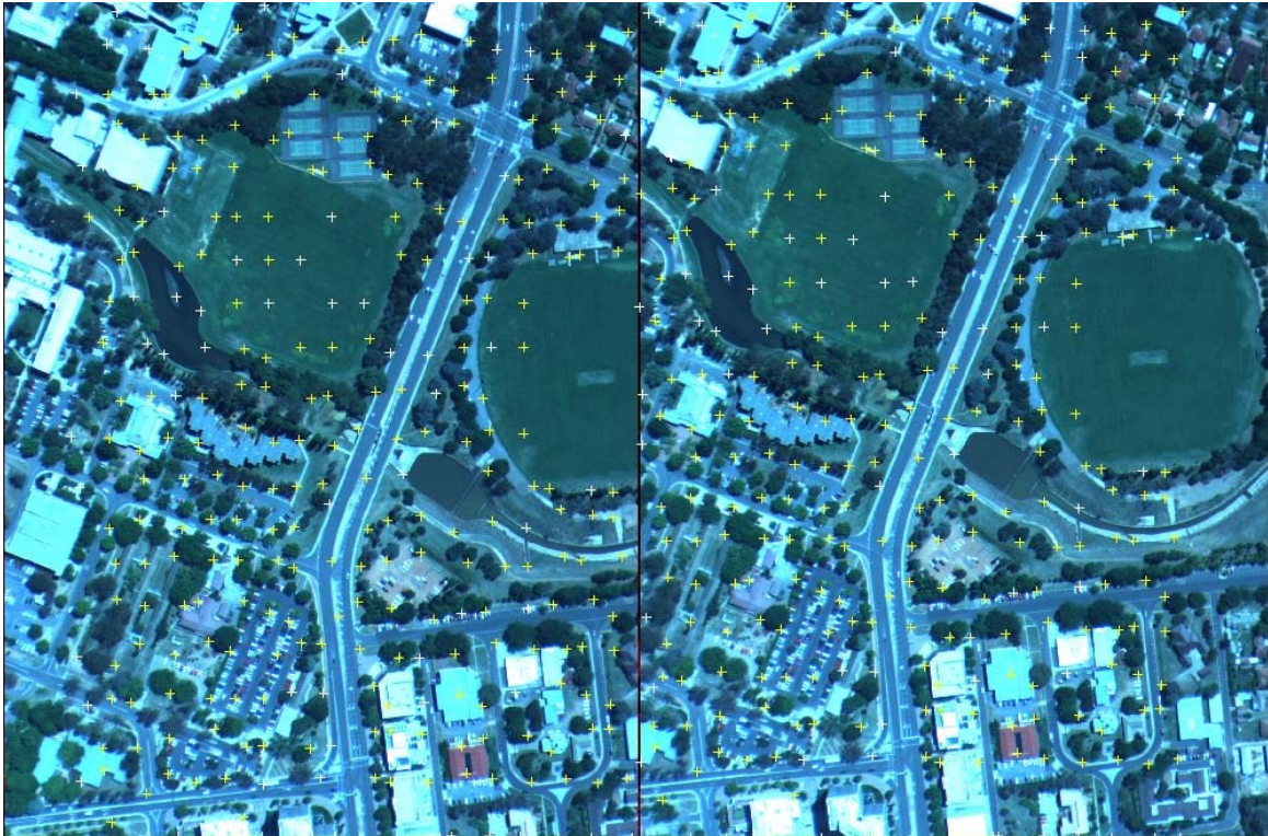
Figure 4-1: The stereo image pair chosen for image orientation experiments. A total of 317 tie points were automatically matched and are shown.
