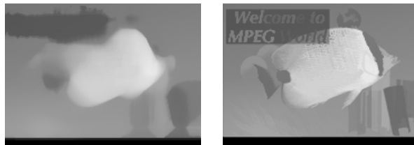
Figure 5. Size filtering with leveling: Left) Median filter with a window of size 15x15 and Right) Self-dual reconstruction of the median filter.
