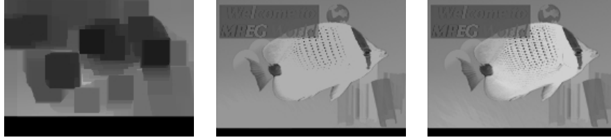
Figure 2. Size filtering with opening by reconstruction: Left) erosion of the original breem image by a flat structuring element of size 10x10, Center) reconstruction of the erosion, and Right) second reconstruction.
