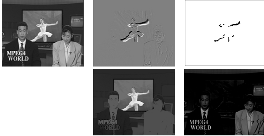
Figure 3. Motion detection of maxima: Top row from left to right: original image, temporal gradient, mask of the marker; Bottom row: anti-extensive reconstruction of the marker, difference between the reconstruction and the original images.
