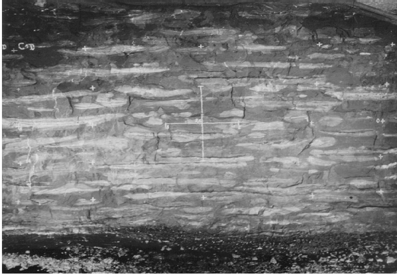
Figure 1. Saint Pierremont mining face (gray bed). The migration of calcite produces nodules which hamper the estimation. Their analysis and modeling as random sets would be the subject of the second study carried out with the texture analyser [SER 68a] .
